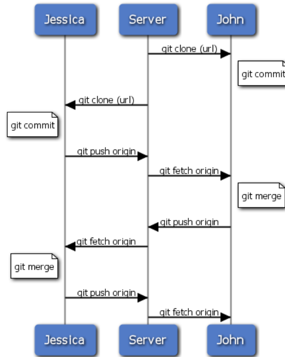
Figure 5.11: General sequence of events for a simple multiple-developer Git workflow.
